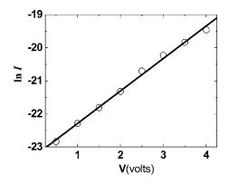
FIG. 2. A typical  $\ln I$ -V curve of the ZnO nanowire at lower bias, corresponding to the curve c in Fig. 1(g).
