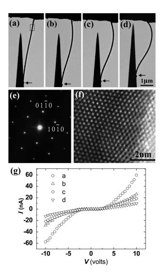
FIG. 1. [(a)-(d)] Sequential TEM images of the four typical bending cases of the ZnO nanowire. (e) Electron diffraction pattern of the framed area in (a), indicating that the nanowire has a wurtzite structure with the  $[01\overline{10}]$  growth direction. (f) The corresponding high-resolution TEM image of the framed area in (a), showing the high-quality single crystal. (g) A series of representative *I*-V curves of the ZnO nanowire, corresponding to the bending cases in (a)–(d).
