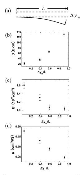
FIG. 3. (a) Simplified scheme of the deflected ZnO naowires. [(b)–(d)] The dependence of resistivity  $\rho$ , electron concentration n, and carrier mobility  $\mu$  on the nanowire bending deflection  $\Delta y_m/L$ .
